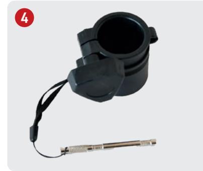
Stick the attachment on the pole of the tripod, and pass the telescope-pole through the attachment into the tripod. Tighten the screw, when the desired height is reached. Save the height with the safety pin.
