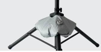
Stick the attachment on the pole of the tripod, and pass the telescope-pole through the attachment into the tripod. Tighten the screw, when the desired height is reached. Save the height with the safety pin.
